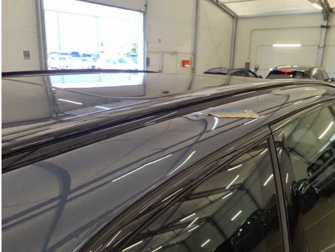
Damage 2: Roof: Roof rail - right side - dent(s) - Smart repair
