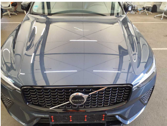
Damage 4: Bonnet: Bonnet - dent(s) - Smart repair
