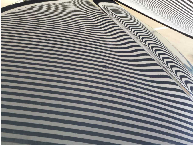
Damage 4: Bonnet: Bonnet - dent(s) - Smart repair
