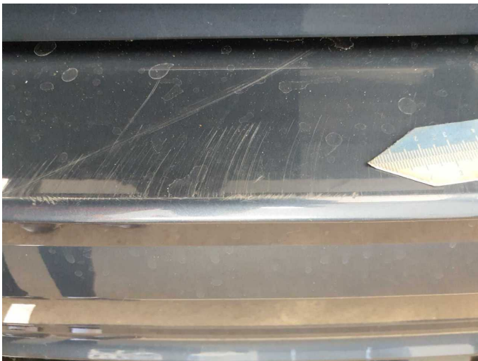
Damage 5: Rear bumper: Rear bumper - Scratch(es) - Paint
