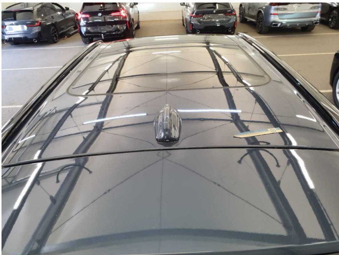
Damage 3: Roof: Roof - dent(s) - Smart repair
