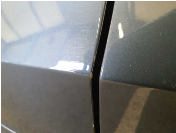
Damage 6: Door - front left side: Door - Dent / paintcoat damage - Paint
