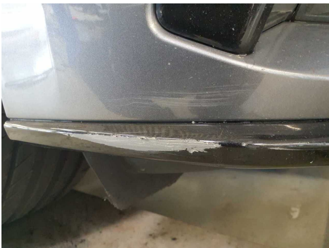
Damage 8: Front bumper: Front bumper - Damaged - repair according to calculation
