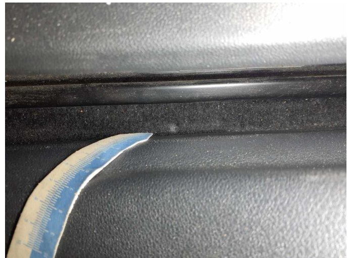
Damage 3: Trim / covers: Floor covering - front left side - Burn hole (cigarettes) - Smart repair
