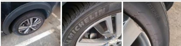
Tyre FL, Out of tolerance, Replace
