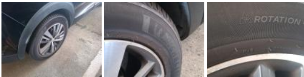
Tyre RL, Out of tolerance, Replace
