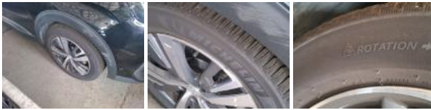
Tyre RR, Out of tolerance, Replace
