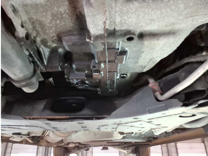
Damage 1: Gearbox: Gearbox - Leaking - Perform diagnosis
