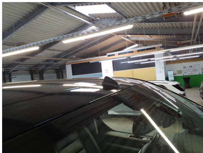
Missing part 2: Roof: Stub aerial - Missing - Replace
