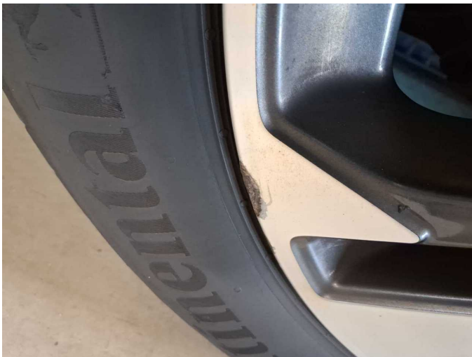
Damage 6: Wheel / tyres: Alloy rim - rear right side (Materialabtrag) - Scratched - Replace
