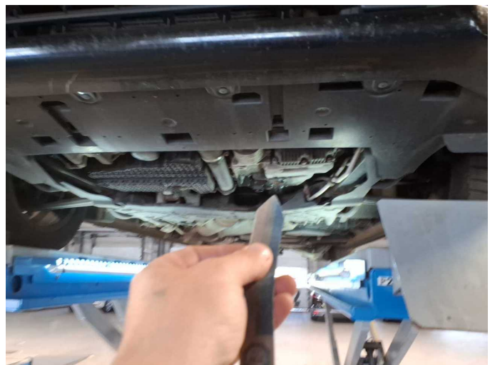
Damage 1: Gearbox: Gearbox - Leaking - Perform diagnosis
