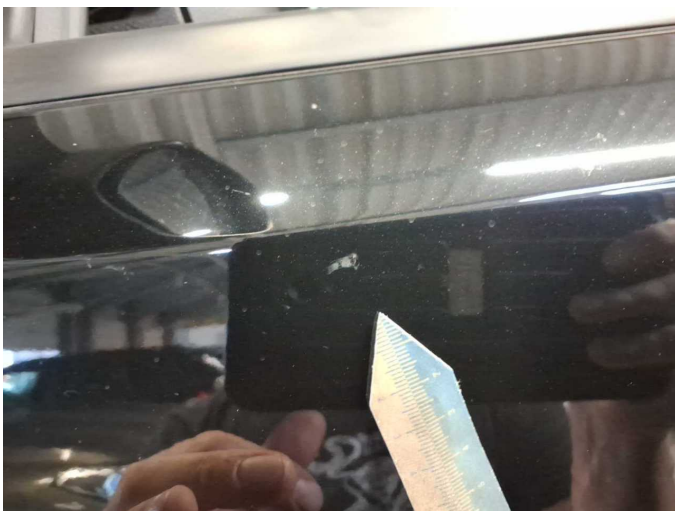
Damage 4: Door - front left side: Door - Dent / paintcoat damage - Smart repair
