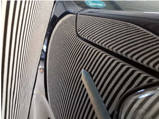
Damage 8: Mudguard - right side: Mudguard - right side - Dent / paintcoat damage - Repair and paint
