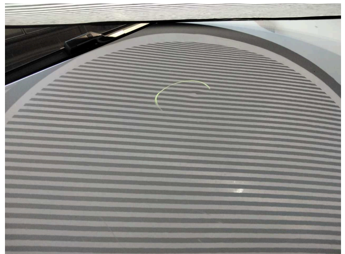
Damage 1: Bonnet: Bonnet - dent(s) - Smooth repair work
