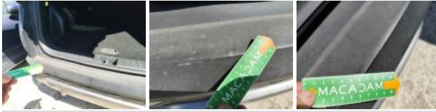
Bumper spoiler Rear, Deformed / Strained, Replace
