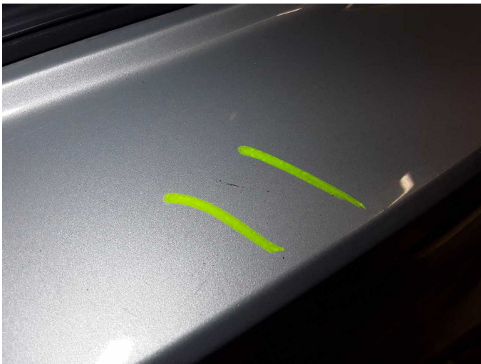
Damage 5: Rear bumper: Rear bumper - Scratch(es) - Paint
