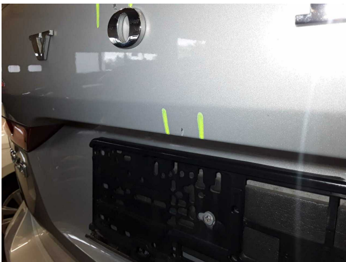
Damage 6: Boot lid / rear door: Boot lid - Scratch(es) - Paint
