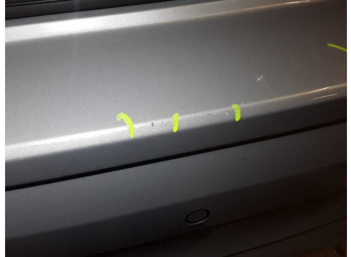
Damage 5: Rear bumper: Rear bumper - Scratch(es) - Paint
