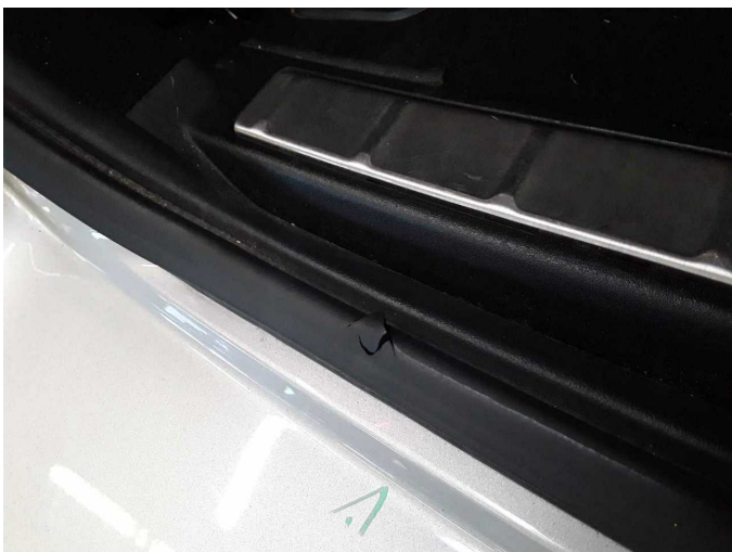
Damage 4: Boot lid / rear door: Seal - Broken / torn - Replace
