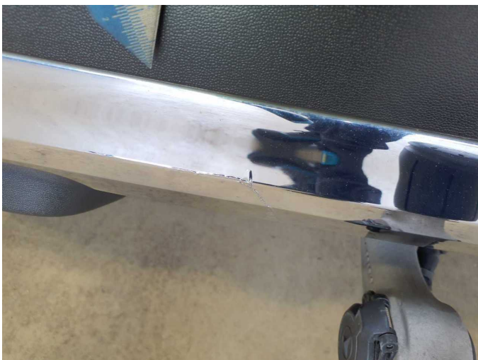
Damage 6: Rear bumper: Spoiler - Scratch(es) - Replace
