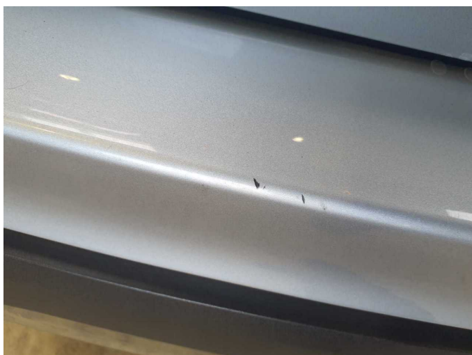
Damage 7: Rear bumper: Rear bumper - Scratch(es) - Paint
