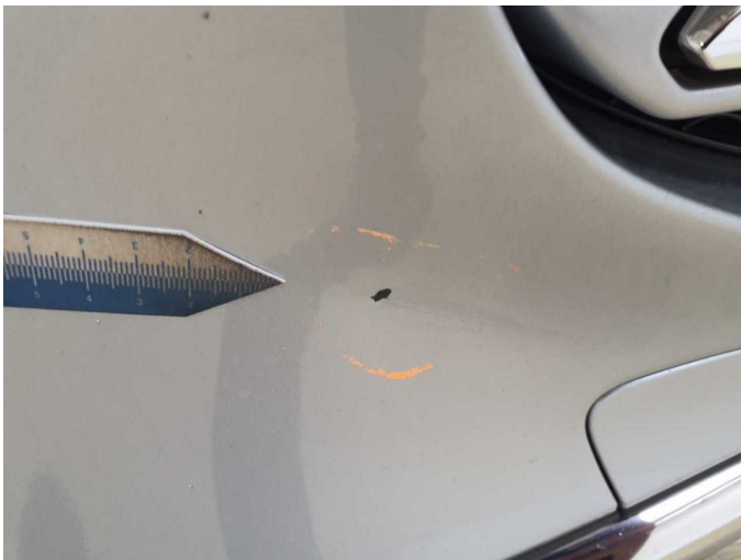
Damage 2: Front bumper: Front bumper - Stone chips - Smart repair
