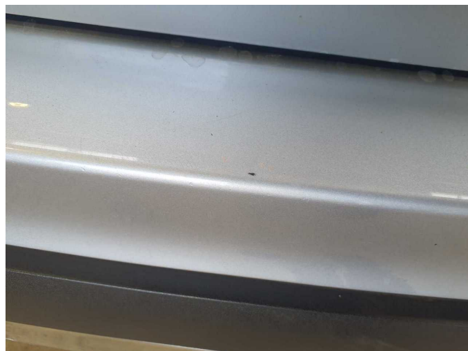
Damage 7: Rear bumper: Rear bumper - Scratch(es) - Paint
