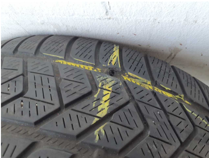
Damage 5: 2nd wheel set: 1 tyre - Leaking - Replace
