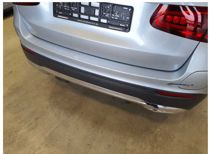
Damage 7: Rear bumper: Rear bumper - Scratch(es) - Paint
