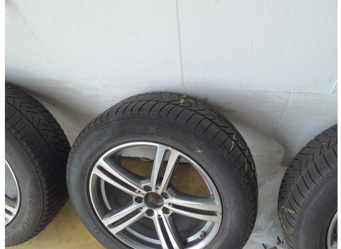
Damage 5: 2nd wheel set: 1 tyre - Leaking - Replace
