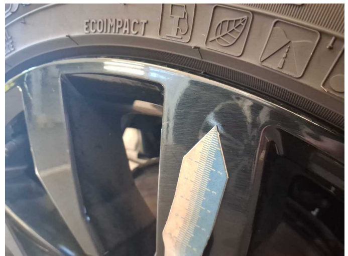
Damage 2: Wheel / tyres: Alloy rim - rear right side - Scratch(es) - Loss in value
