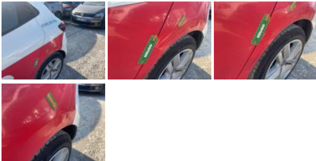
Door RL, Dent(s), Repair and paint (complete)
