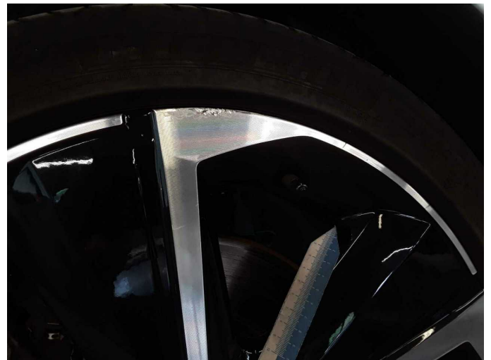
Damage 5: Wheel / tyres: Alloy rim - front left side - Scratched - Loss in value
