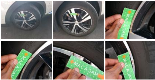
Tyre RL, Out of tolerance, Replace
