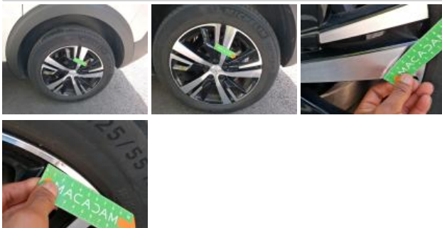
Tyre RR, Out of tolerance, Replace
