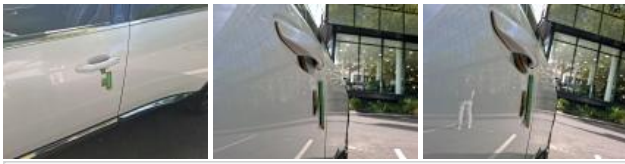
Door RL, Dent(s), Repair and paint (complete)
