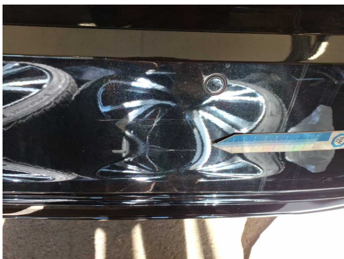
Damage 4: Rear bumper: Rear bumper - Scratched - Paint
