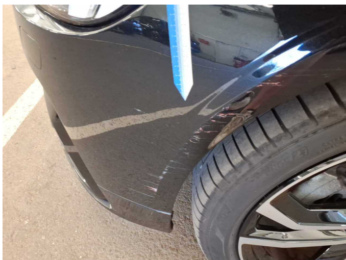
Damage 9: Front bumper: Front bumper - Scratched - Paint
