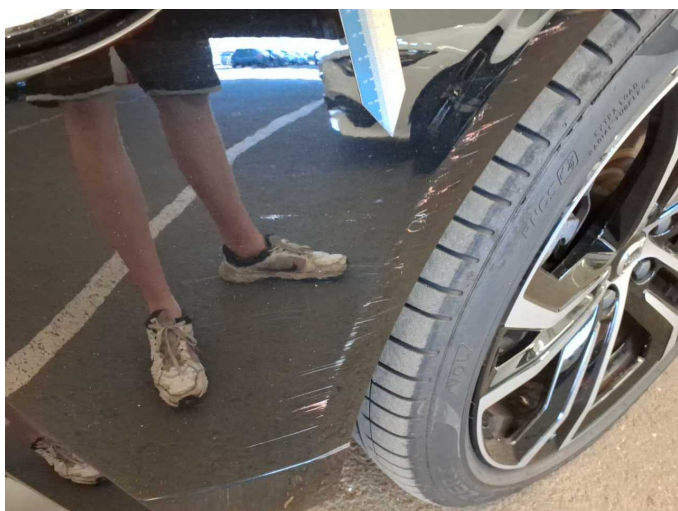
Damage 9: Front bumper: Front bumper - Scratched - Paint
