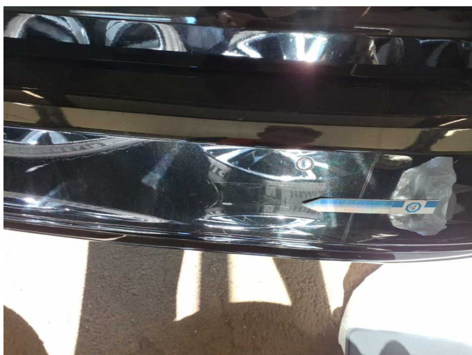
Damage 4: Rear bumper: Rear bumper - Scratched - Paint
