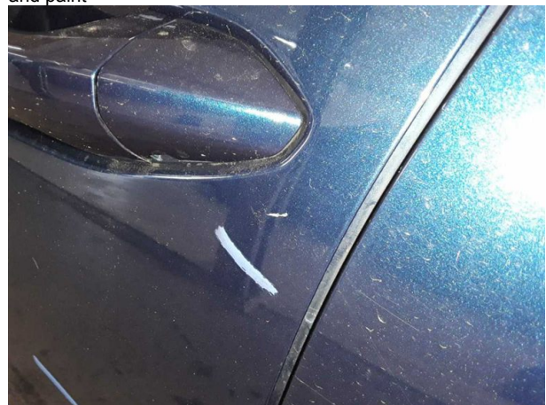
Damage #8: Door - front left side: Door - Scratched - Repair and paint
