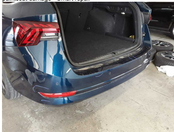
Damage #7: Rear bumper: Rear bumper - Scratched - Repair and paint
