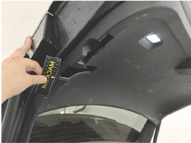
Shutter / cover Missing Replace Interior
