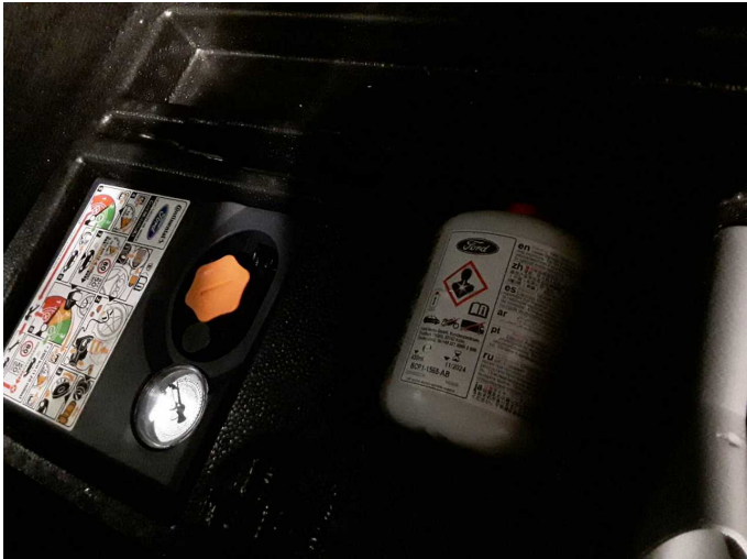
Damage 1: Equipment: Tirefit filler - Expired - Replace
