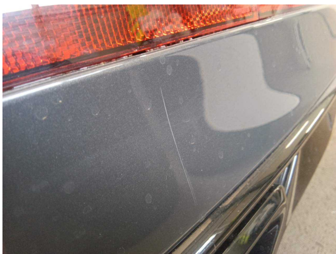
Damage 3: Rear bumper: Rear bumper - Scratch(es) - Paint
