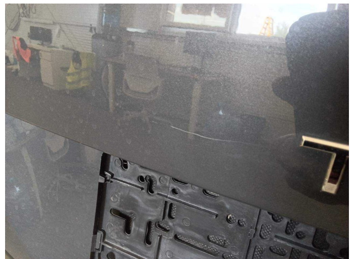
Damage 6: Boot lid / rear door: Boot lid (& Lackschaden) - Dent / paintcoat damage - Repair and paint
