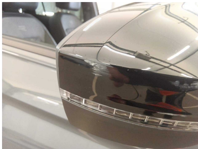
Damage 2: Wing mirror - right side: Cap - Scratched - Replace
