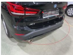
6 - Bumper R - Dent(s) and scratch(es)
