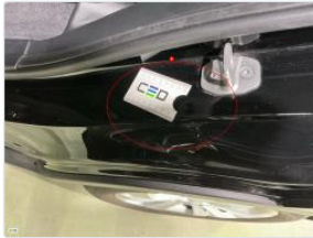
5 - Wing RL - Dent(s) and scratch(es)
