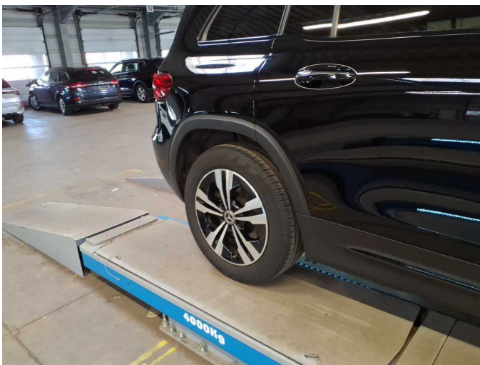
Damage 7: Wheel / tyres: Tyre - rear right side (Flanke,nicht fahrbereit) - Damaged - Replace
