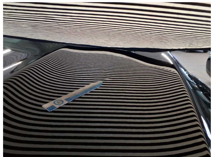
Damage 2: Bonnet: Bonnet - dent(s) - Smooth repair work
