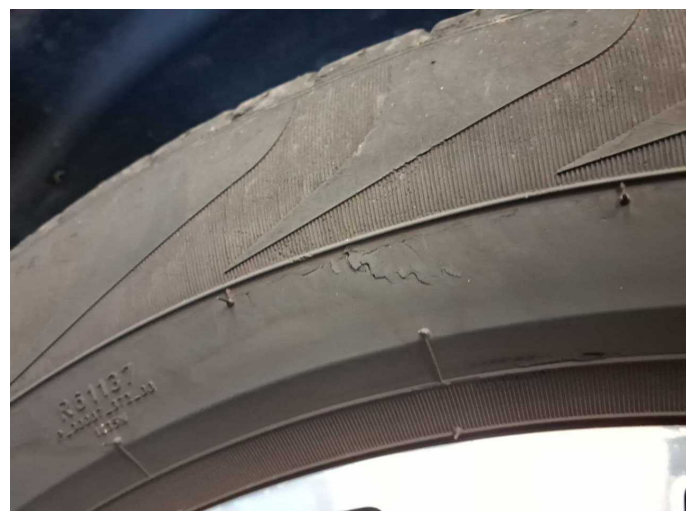
Damage 8: Wheel / tyres: Tyre - front right side (Flanke,nicht fahrbereit) - Damaged - Replace
