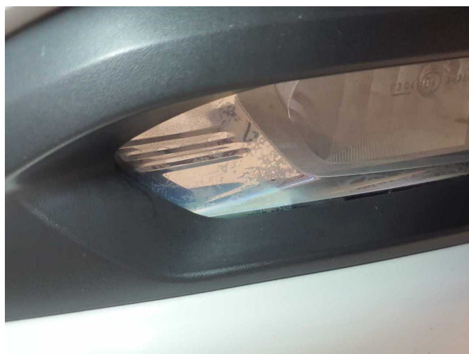
Wear and tear 2: Fog lamp: Fog lamp - front left side - Scratch(es) - No deduction
