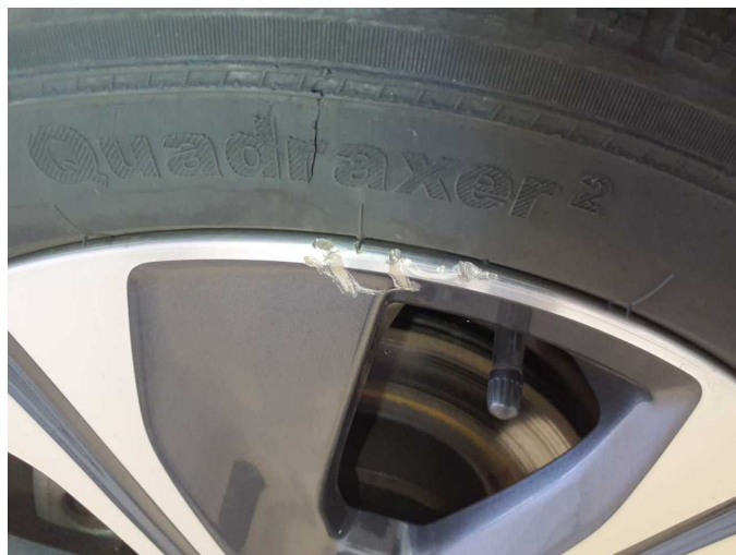
Damage 16: Wheel / tyres: Alloy rim - rear right side - Scratch(es) - Replace
