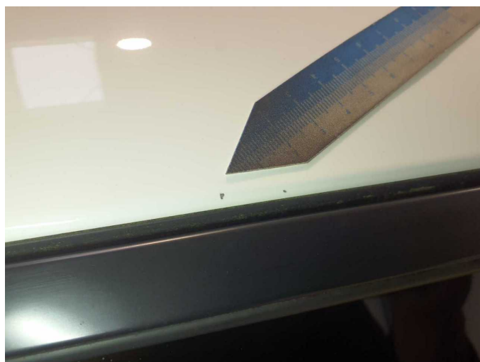
Damage 11: Roof: Roof rail - right side - Scratch(es) - Smart repair
