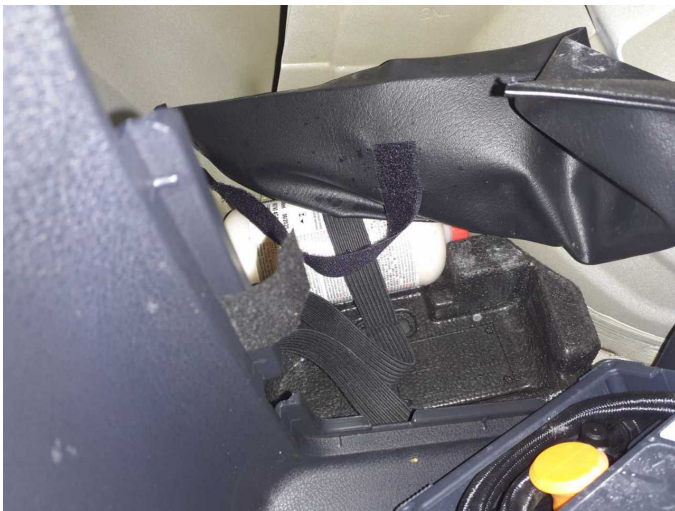
Damage 3: Equipment: Tirefit filler - Expired - Replace
