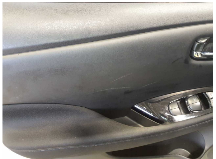
Damage 5: Trim / covers: Door trim - front left side - Scratch(es) - Loss in value
