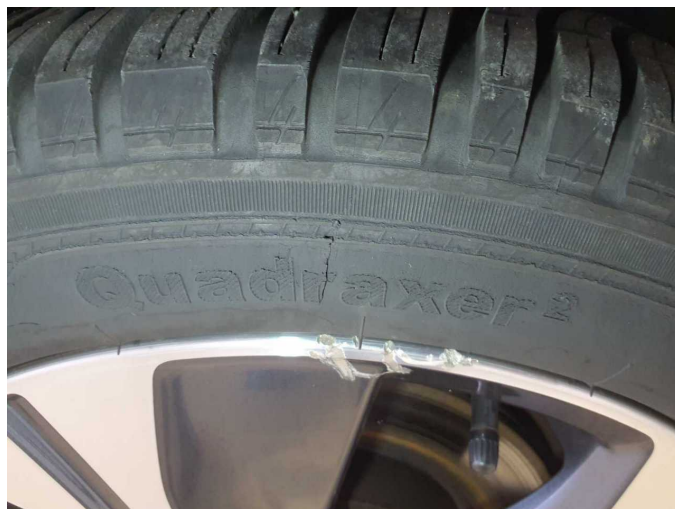
Damage 12: Wheel / tyres: Tyre - rear right side (nicht fahrbereit) - Broken / torn - Replace
