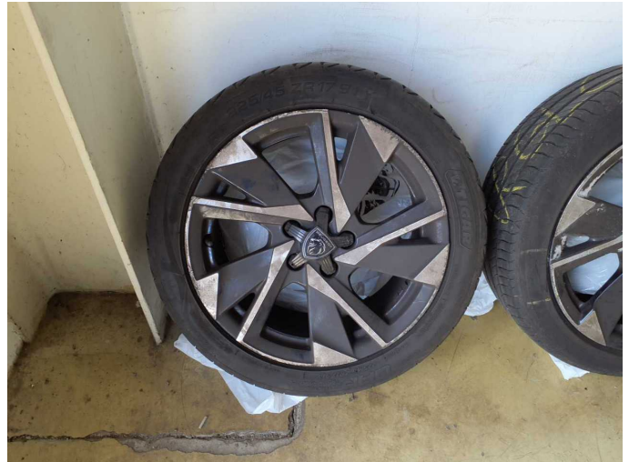
Damage 12: 2nd wheel set: 1 alloy rim - Scratch(es) - Replace
