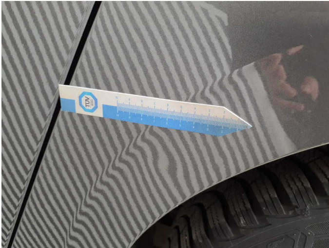
Damage 7: Side panel - rear left side: Side panel - dent(s) - Smart repair
