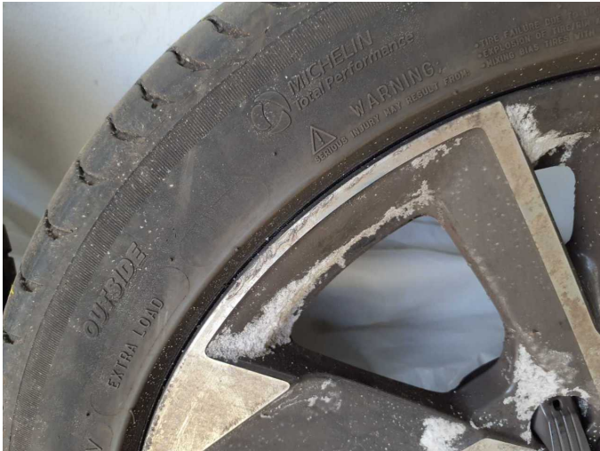
Damage 11: 2nd wheel set: 1 alloy rim - Scratch(es) - Replace
