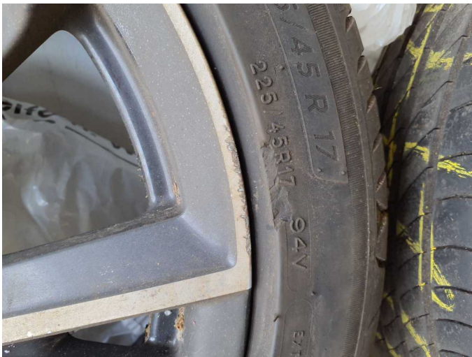
Damage 10: 2nd wheel set: 1 alloy rim - Scratch(es) - Replace
