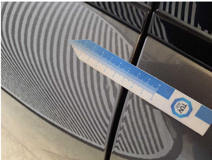
Damage 5: Door - rear right side: Door - Dent / paintcoat damage - Smart repair
