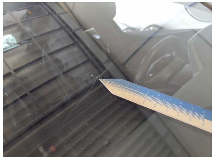
Damage 16: Vehicle glazing: Windscreen - Broken / torn - Replace
