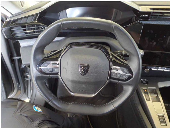
Damage 15: Steering system: Steering wheel (Airbag) - Porous / cracked - Replace
