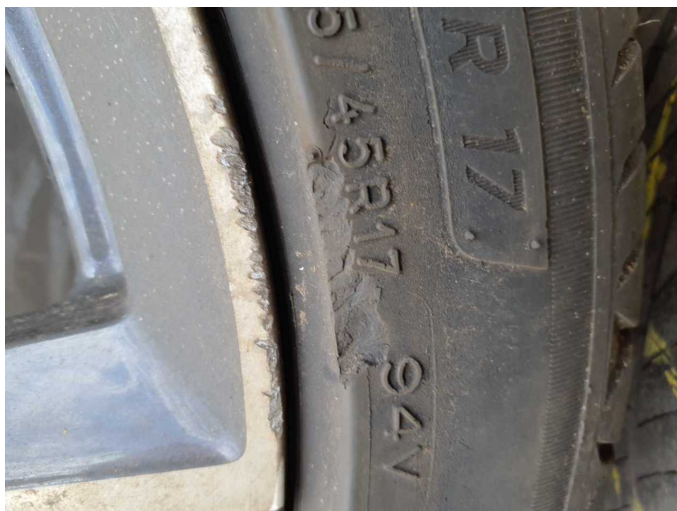
Damage 13: 2nd wheel set: 3 tyres - Broken / torn - Replace
