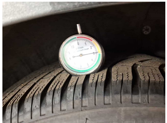
Damage 4: Wheel / tyres: Tyre - rear right side - Does not meet the leasing specifications - Replace
