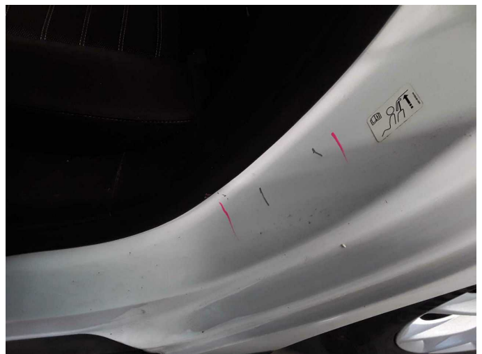
Damage 6: Body: D-pillar - left side - Dent / paintcoat damage - Smart repair
