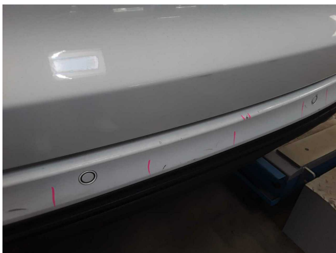
Damage 10: Rear bumper: Rear bumper - Scratch(es) - Paint
