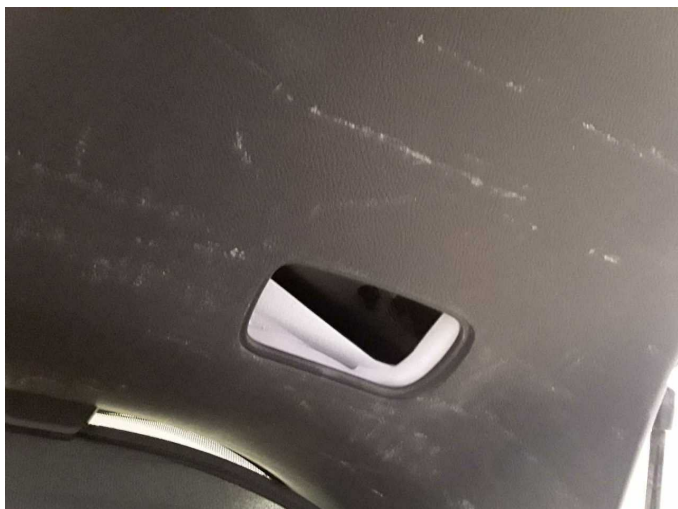
Damage 9: Boot lid / rear door: Trim - standard - lower (+ unvollständig) - Scratched - Replace
