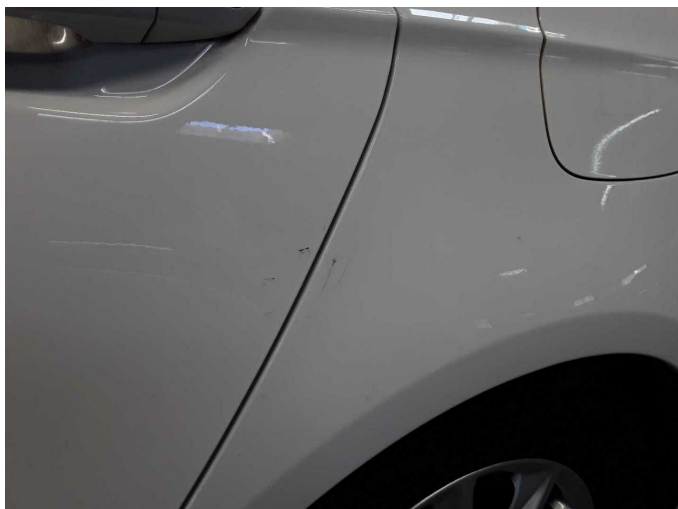
Damage 7: Body: Body (Klebereste) - Glued / labelled - De-glue / neutralise
