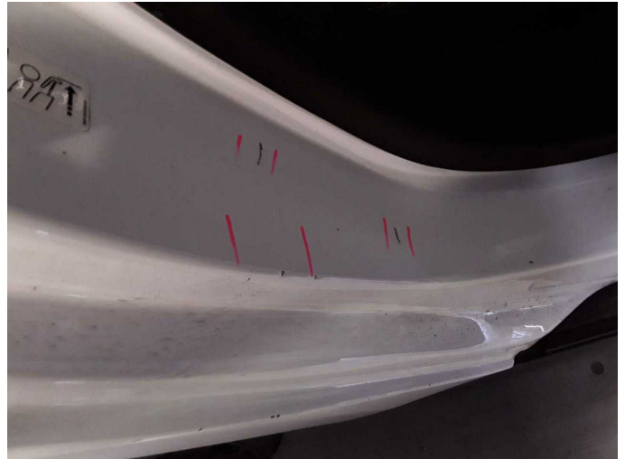
Damage 5: Body: C-pillar - right side - Dent / paintcoat damage - Smart repair
