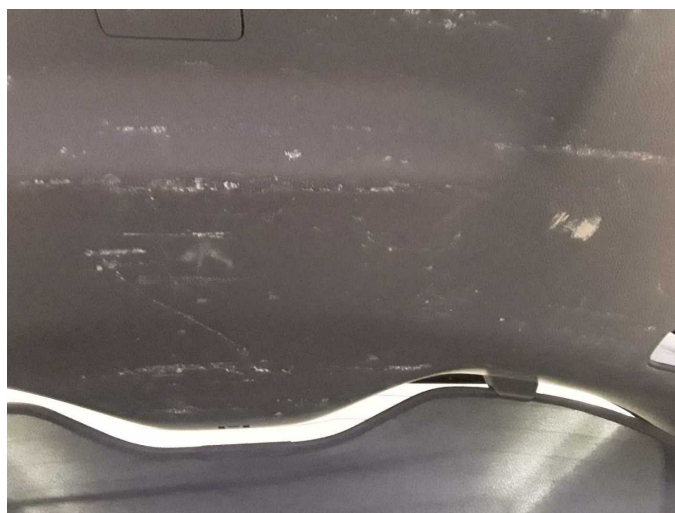
Damage 9: Boot lid / rear door: Trim - standard - lower (+ unvollständig) - Scratched - Replace
