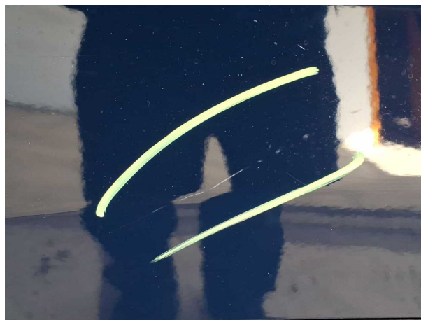
Damage #2: Side panel - rear left side: Side panel - Scratched - Cover / polish
