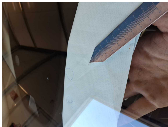
Damage 7: Vehicle glazing: Windscreen (Beheizbare Frontscheibe) - Stone chips - Replace
