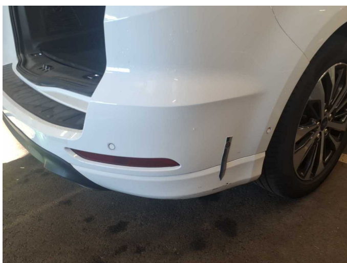
Damage 5: Rear bumper: Rear bumper - Scratch(es) - Paint
