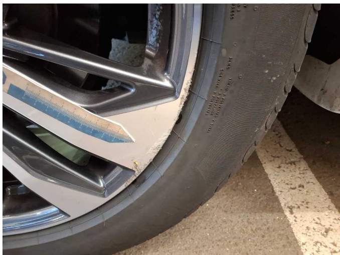
Damage 4: Wheel / tyres: Alloy rim - rear right side (Materialabtrag) - Scratch(es) - Replace
