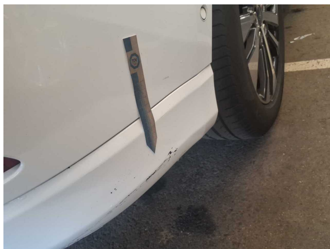
Damage 5: Rear bumper: Rear bumper - Scratch(es) - Paint
