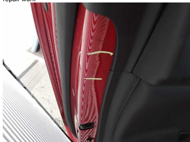
Damage #10: Door - rear left side: Door - dent(s) - Smooth repair work
