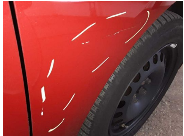
Damage #11: Mudguard - right side: Mudguard - right side - Scratched - Repair and paint
