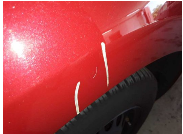
Damage #3: Mudguard - left side: Mudguard - left side - Scratched - Smart repair
