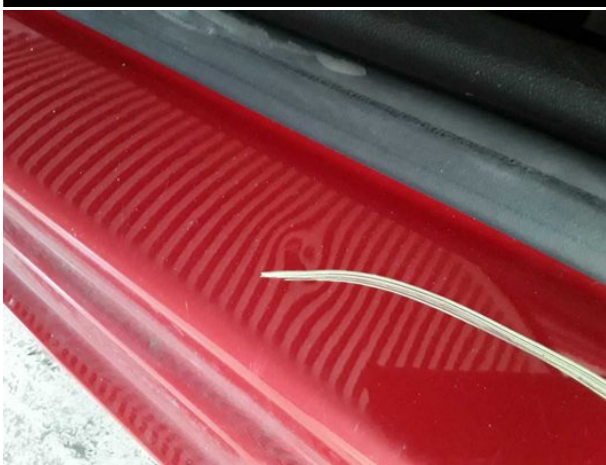
Damage #8: Sill - left side: Sill - Dent / paintcoat damage - Smart repair
