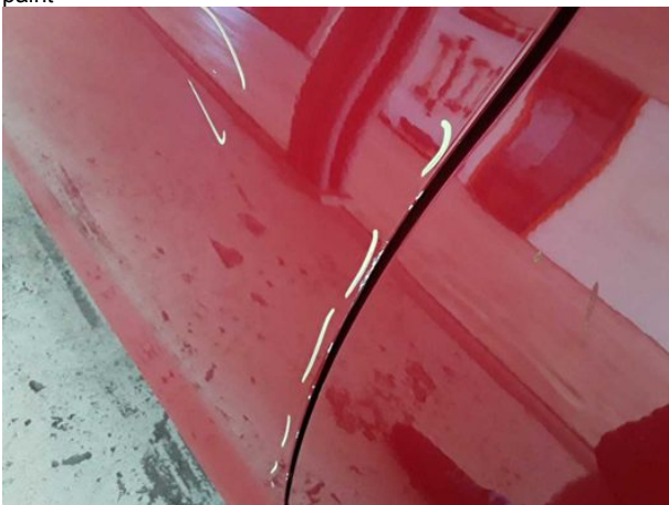
Damage #13: Door - front left side: Door - Scratched - Repair and paint
