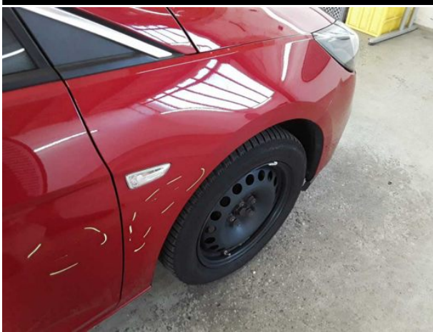
Damage #11: Mudguard - right side: Mudguard - right side - Scratched - Repair and paint
