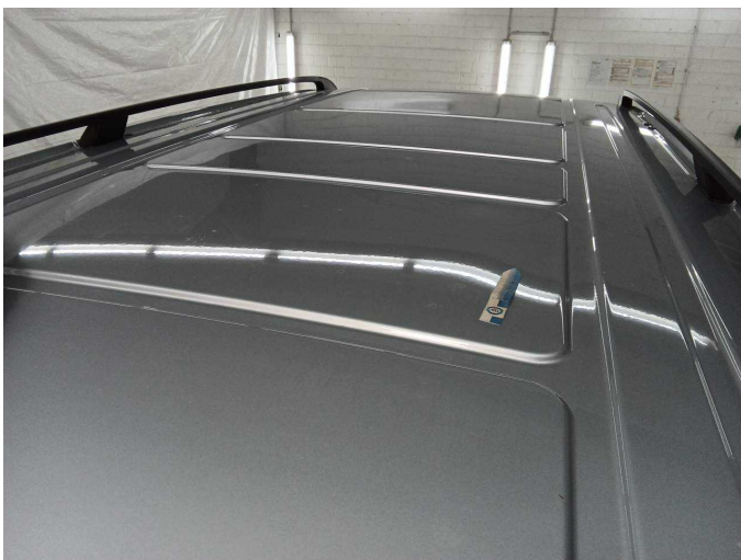
Damage 1: Roof: Roof - dent(s) - Smooth repair work
