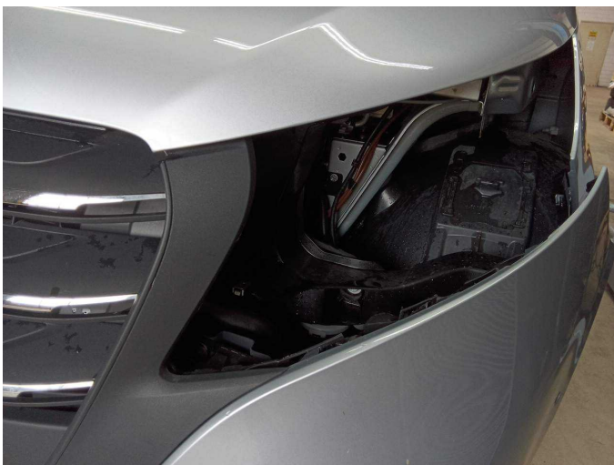
Damage 6: Headlight: Headlight - left side (+ rechts) - Missing - Replace
