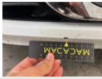
Wing RR, Dent(s) and scratch(es), Repair and paint (complete)
