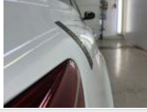
Wing RR, Dent(s) and scratch(es), Repair and paint (complete)
