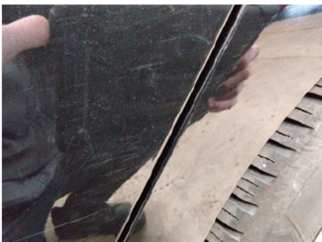
Tür / Hinten Links / Kratzer
