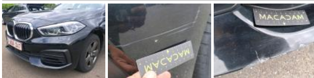
Bumper F, Dent(s) and scratch(es), Repair and paint (complete)
