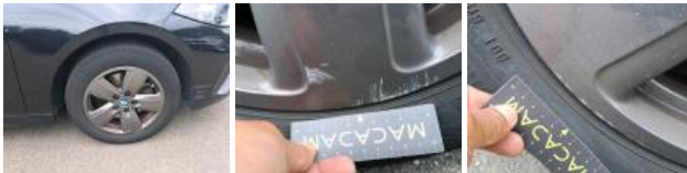
Tyre FR, Tear, Replace
