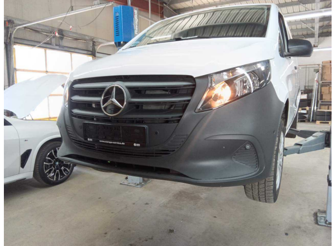
Damage 5: Front bumper: Front bumper - Malposition - Un- / install
