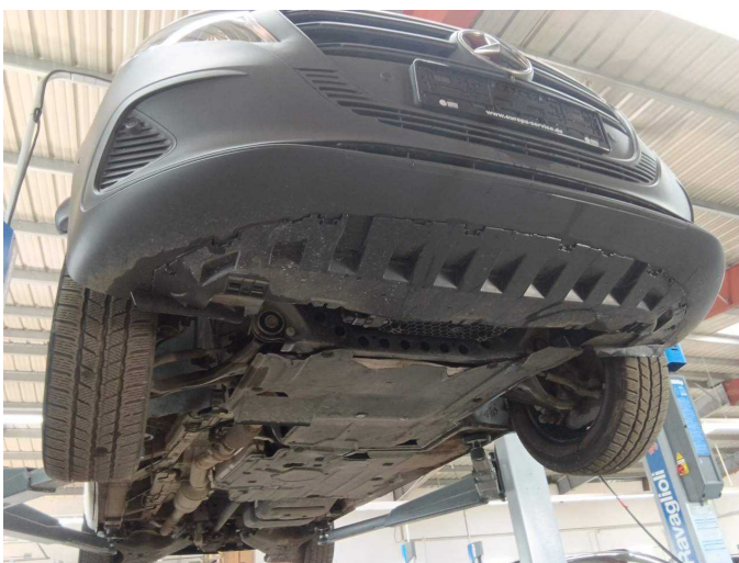
Damage 1: Body: Underbody panelling - Scratch(es) - Replace
