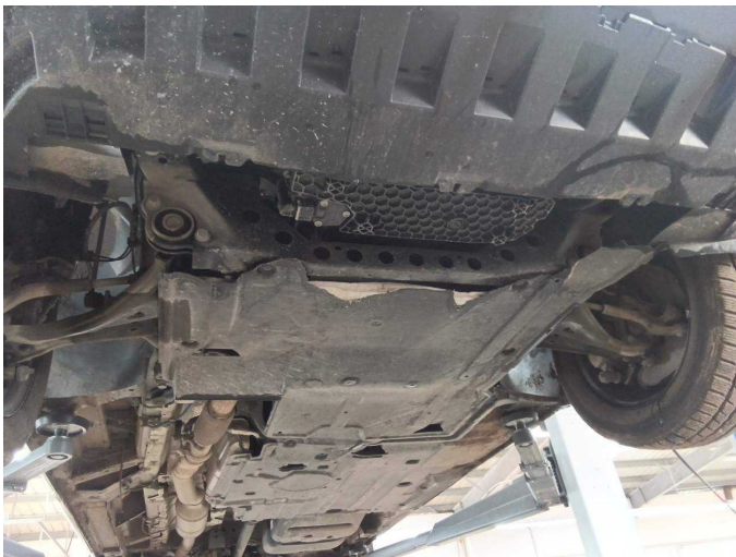
Damage 3: Engine: Engine cowling - lower - Broken / torn - Replace
