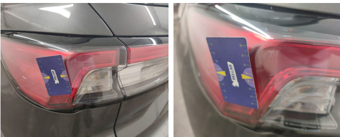
Light / Rear left / Replace-scratch
