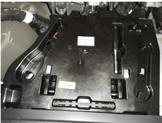
Missing part 1: Equipment: Vehicle tool kit - Missing - Replace
