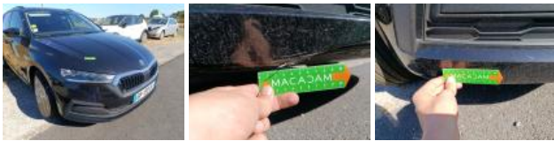
Door FR, Dent(s), Repair and paint (complete)
