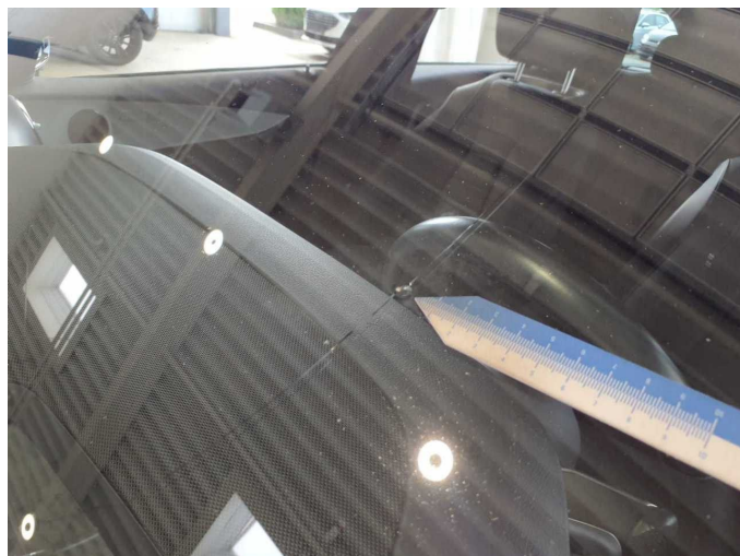
Damage 10: Vehicle glazing: Windscreen - Broken / torn - Replace
