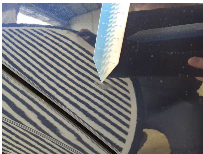
Damage 7: Door - rear right side: Door (Sprühnebel) - Paint defect - Repair and paint
