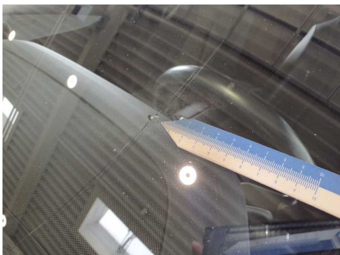
Damage 10: Vehicle glazing: Windscreen - Broken / torn - Replace
