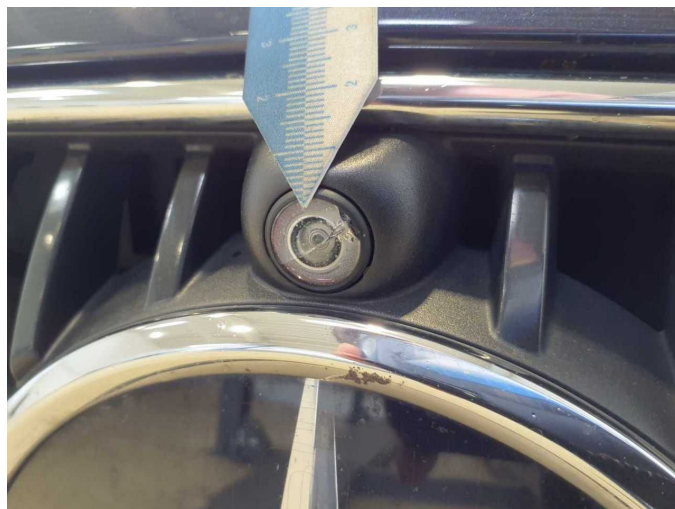
Damage 6: Electronic systems: Front camera - Broken / torn - Replace
