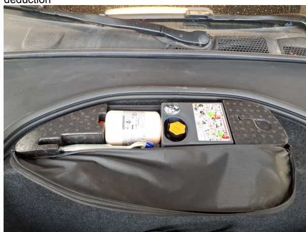
Damage #3: Equipment: Tirefit filler - Expired - Replace
