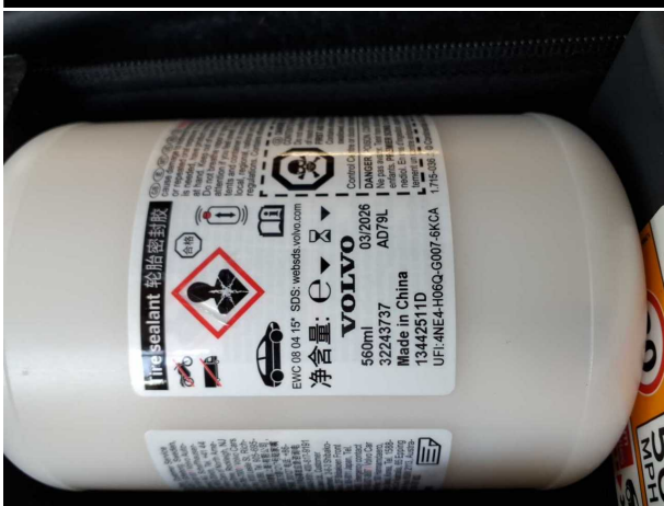
Damage #3: Equipment: Tirefit filler - Expired - Replace
