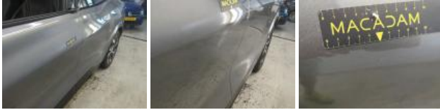
Door RL, Dent(s), Repair and paint (complete)
