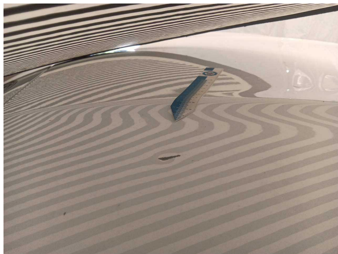
Damage 4: Bonnet: Bonnet - Dent / paintcoat damage - Paint
