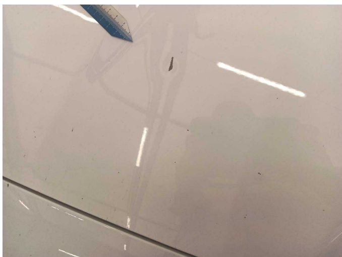
Damage 4: Bonnet: Bonnet - Dent / paintcoat damage - Paint
