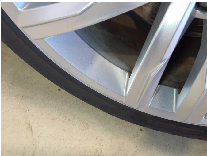
Damage 11: Wheel / tyres: Alloy rim - rear left side (Sichtbar Bearbeitet) - Unprofessionally repaired - Replace
