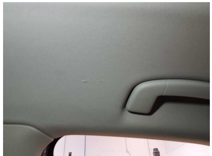
Damage 3: Trim / covers: Roof lining - Scratch(es) - Smart repair
