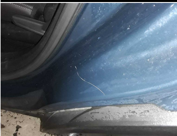
Damage #7: Side panel - rear left side: Sill - Scratched - Repair and paint
