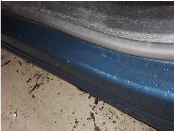
Damage #7: Side panel - rear left side: Sill - Scratched - Repair and paint
