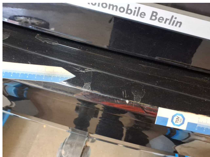
Damage 17: Rear bumper: Rear bumper - Scratch(es) - Paint
