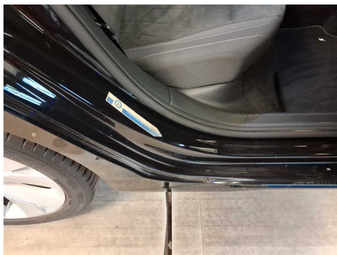
Damage 10: Side panel - rear right side: Sill - Scratch(es) - Smart repair
