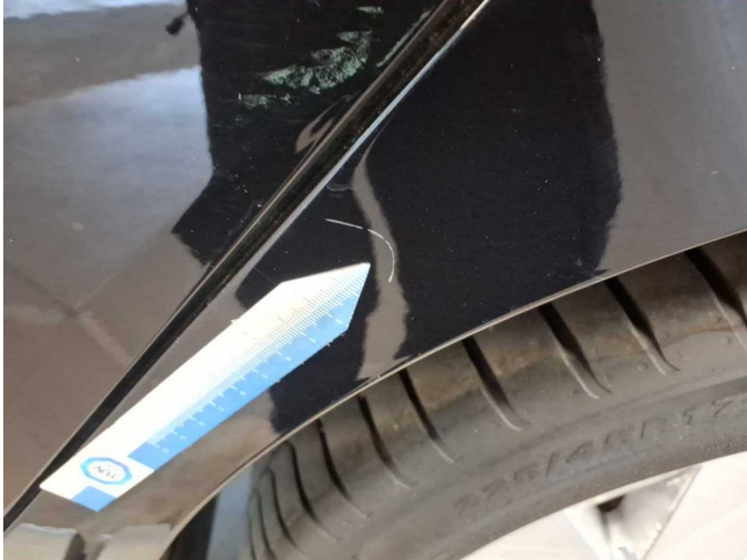
Damage 11: Side panel - rear left side: Side panel - Scratch(es) - Smart repair
