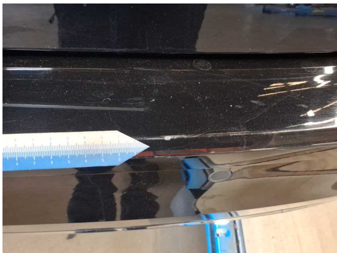
Damage 17: Rear bumper: Rear bumper - Scratch(es) - Paint
