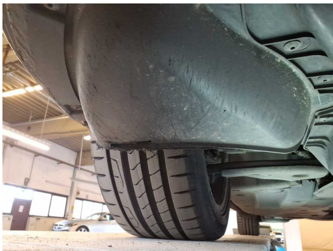
Wear and tear 7: Body: Wheel well - front right side (Radhausschale unterhalb) - Scratched - No deduction
