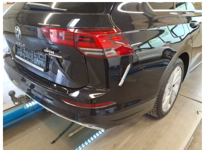
Damage 17: Rear bumper: Rear bumper - Scratch(es) - Paint
