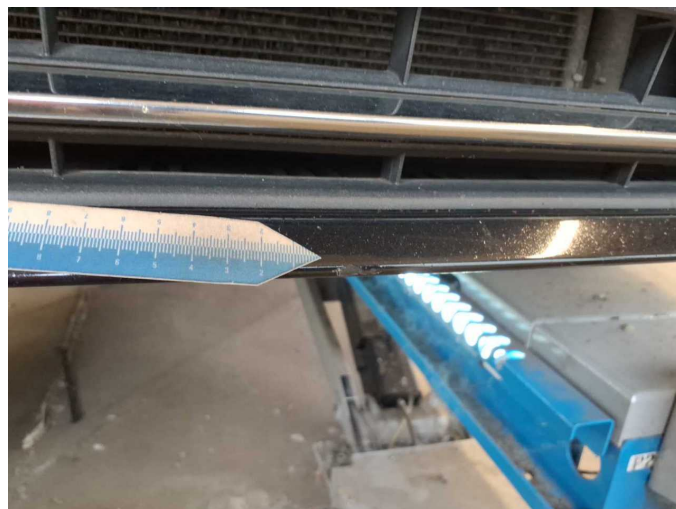
Damage 20: Front bumper: Front bumper (+ Steinschläge) - Scratch(es) - Paint
