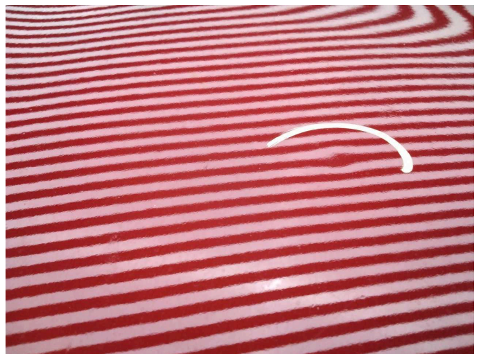
Damage 6: Bonnet: Bonnet - Dent / paintcoat damage - Paint
