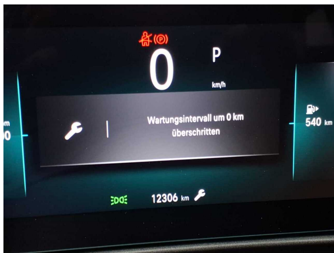
Damage 5: Misc.: Inspection / maintenance - Due - Replace
