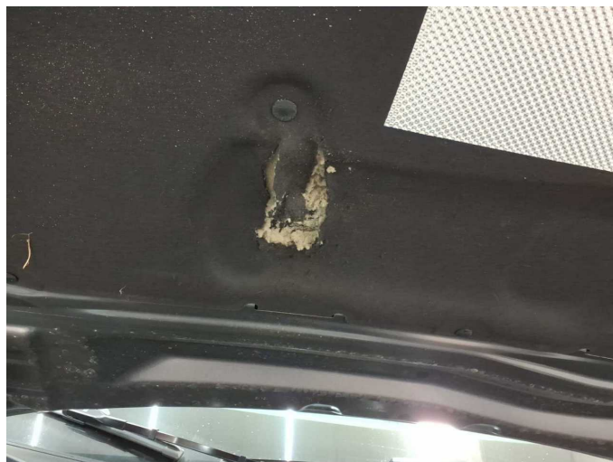
Damage 3: Bonnet: Insulation lining - Holes - Replace
