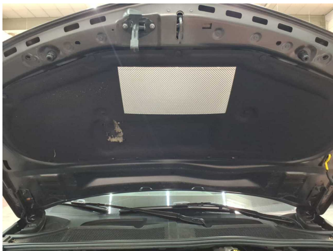
Damage 3: Bonnet: Insulation lining - Holes - Replace
