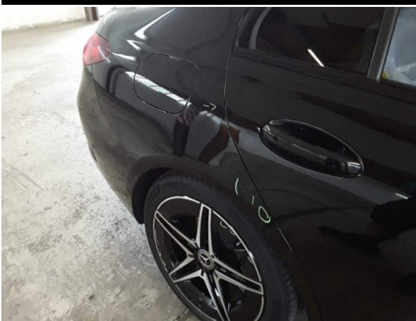
Damage #13: Side panel - rear right side: Side panel - Dent / paintcoat damage - Repair and paint
