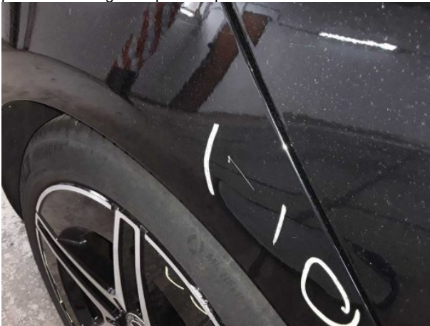
Damage #13: Side panel - rear right side: Side panel - Dent / paintcoat damage - Repair and paint
