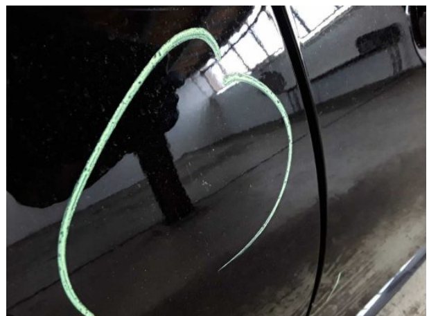
Damage #9: Door - rear right side: Door - Dent / paintcoat damage - Smart repair
