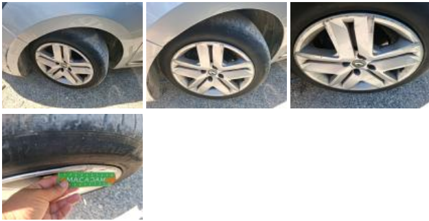
Tyre FR, Out of tolerance, Replace
