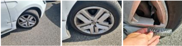
Tyre FR, Out of tolerance, Replace
