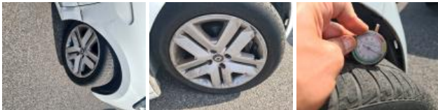
Tyre FL, Out of tolerance, Replace
