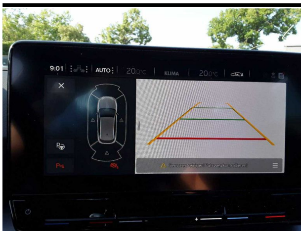
Damage #5: Electronic systems: Rear view camera - Damaged - Replace
