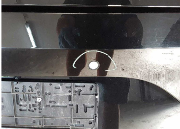
Damage #6: Electronic systems: Parking assistance (4 Stück falscher Farbton) - Differs from the original configuration - Replace
