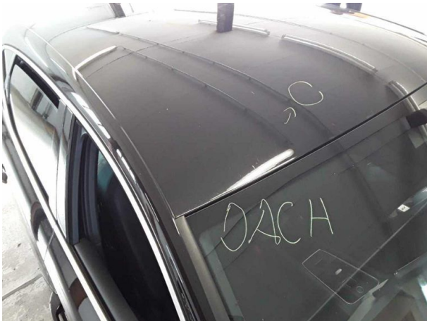
Damage #1: Roof: Roof - dent(s) - Smooth repair work
