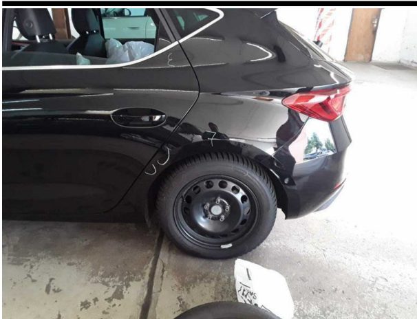
Damage #4: Side panel - rear left side: Side panel - dent(s) - Smooth repair work
