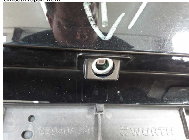
Damage #5: Electronic systems: Rear view camera - Damaged - Replace
