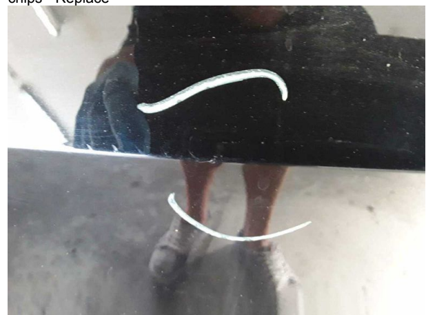
Damage #8: Rear bumper: Rear bumper - Scratched - Paint
