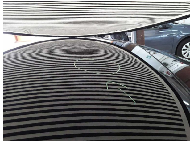
Damage #1: Roof: Roof - dent(s) - Smooth repair work
