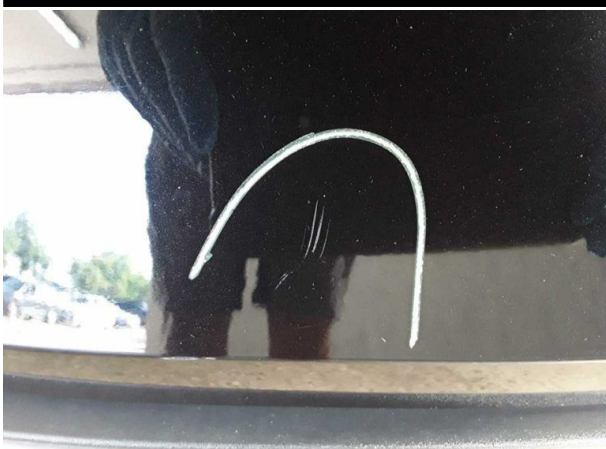
Damage #8: Rear bumper: Rear bumper - Scratched - Paint
