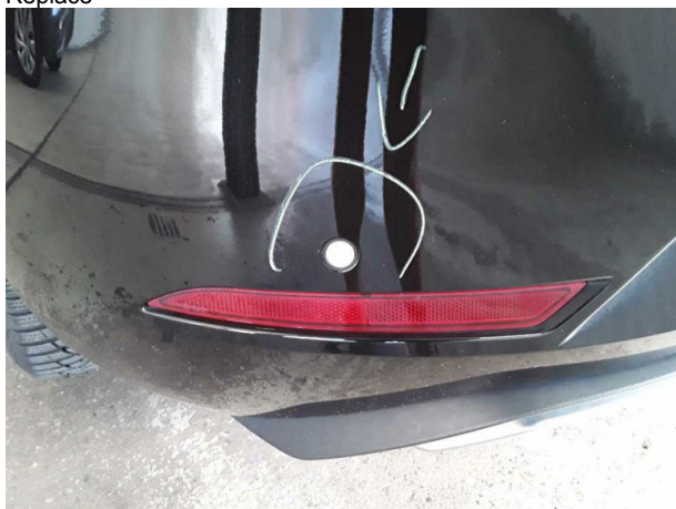
Damage #6: Electronic systems: Parking assistance (4 Stück falscher Farbton) - Differs from the original configuration - Replace
