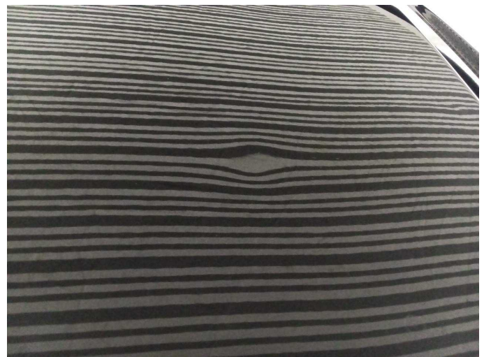
Damage 4: Roof: Roof (4 Dellen) - dent(s) - Smooth repair work
