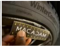
Tyre RR, Tear, Replace
