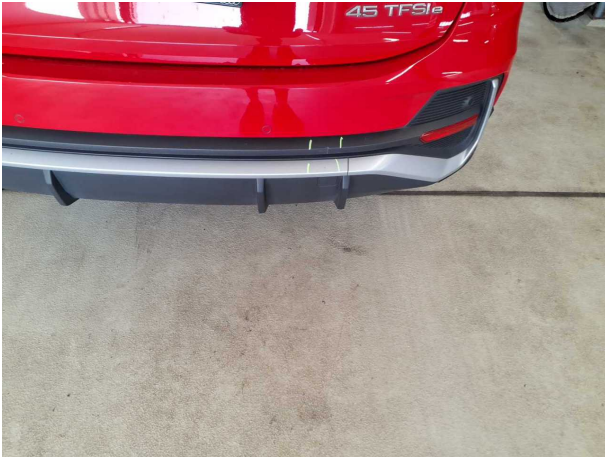
Damage #2: Rear bumper: Spoiler - Deformed - Replace
