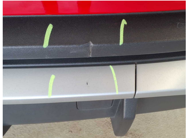
Damage #2: Rear bumper: Spoiler - Deformed - Replace
